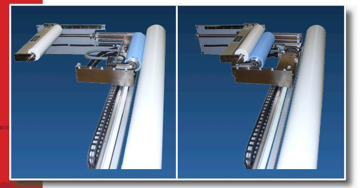
Polymag<sup>®</sup> Tek's Backing Roll Cleaner uses a traversing Contact Cleaning Roll to remove contaminants from the backing roll. After removing contaminants from the backing roll, the contact cleaning roll traverses to a home location, where it transfers the collected contaminates to an adhesive tape roll for permanent elimination.
